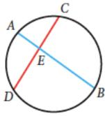
The formula used to determine the radius of the yaw mark arc is derived from a geometric relationship about two intersecting chords in a circle. In the figure, chords  $\overline{AB}$  and  $\overline{CD}$  intersect at point E in the circle. The product of the two segment lengths making up chord  $\overline{AB}$ ,  $AE \times EB$ , is equal to the product of the two segment lengths making up chord  $\overline{CD}$ ,  $CE \times ED$ .
