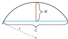
The center of the chord is located and a perpendicular line segment is drawn from that center to the arc, creating a right angle. This short line segment is the middle ordinate.
